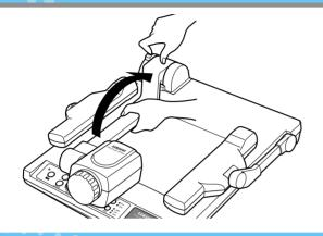
Adjust the angle of the lamps properly.
