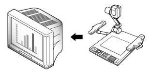
■ Connect a TV, PC monitor or Projector to this presenter to display the projected image using the AV cables, S-video cable or PC monitor cable.
