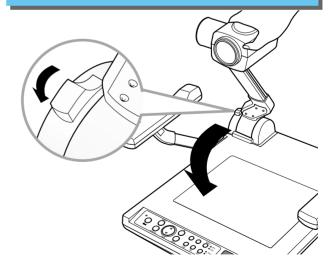
5 Fold the lamps on both sides completely.
