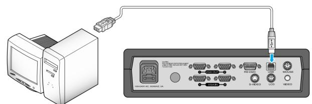
Connect to the USB port on your PC, then install the supplied SDP-6500 program.
