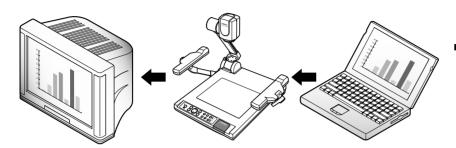
If you connect computer through VGA IN port, you can receive video signal from the computer.
