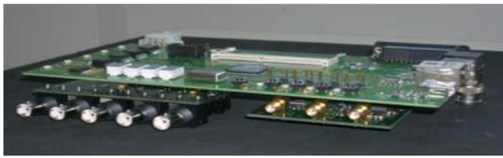
ICTP RVI hardware setup for a reconfigurable virtual instrumentation system.
